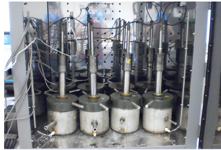
Several fully assembled VCMDs inside an oven used for conducting this test at a particular temperature in the Center for Infrastructure Renewal’s Concrete Innovation Laboratory.
